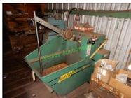
**61 Precision Husky Model 6K 6-Knife Tub Knife Sharpener Grinder**
